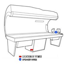
\*Owner is responsible for all wiring up to the terminal block connection inside the device. As well as ensuring the wire is properly sized for the amp draw and breaker selection per the electrical code in their area.
